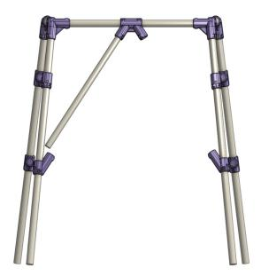
Figure A7. Connected first angled support.
