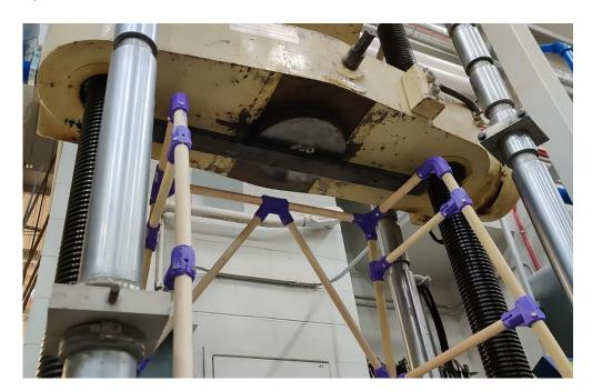
Figure 5. Testing distributed load that replicates the span of a fists on the walker.
