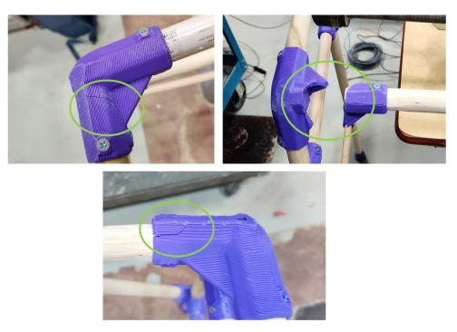
**Figure 11.** Sample images of failure occurring at the 3D-printed Ang 3 Connector part after horizontal walker testing.
